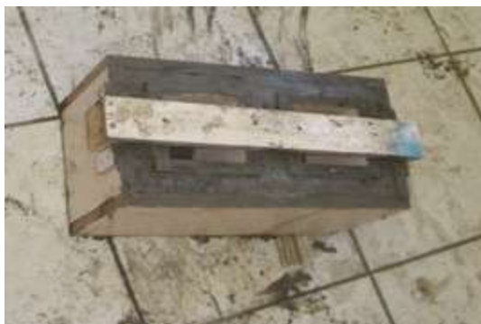
Fig.6 Details of mold of the ferrocement block
