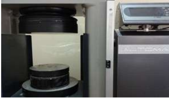
Fig.8 Testing machine for control specimens (compression test)
