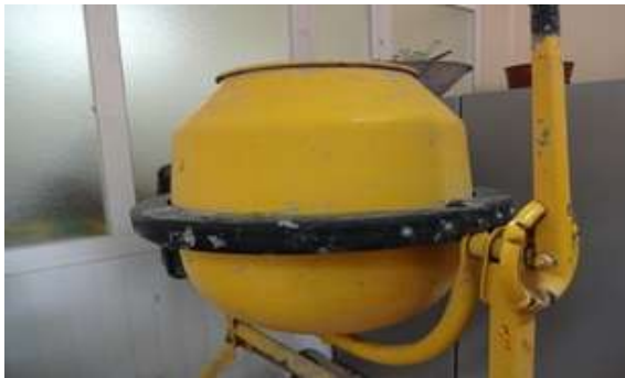
Fig.4 Tilting pan type mixer
