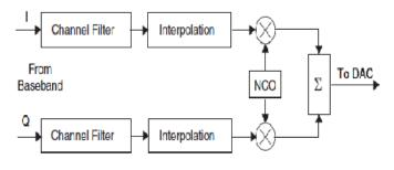
Figure 8- DUC Block Diagram [1]
