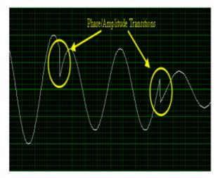
Fig2. Phase and Amplitude Transitions in an Unfiltered Modulated Signal[8]
