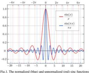
Fig.1. The normalized (blue) and unnormalized (red) sinc functions [7]
