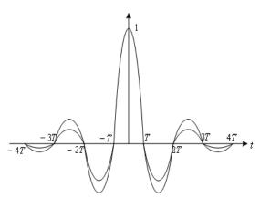
Figure 6- Impulse response of RC filter
