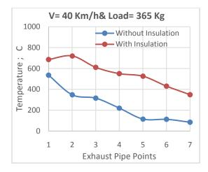
Fig. (11) Temperature distribution at 40 Km/h car speed and load of 365 Kg
