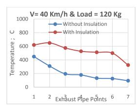
Fig. (10) Temperature distribution at 40 Km/h car speed and load of 120 Kg.
