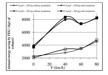
Fig. (15) Annual energy saving by TEG / (kg/s of exhaust) for different car velocities and loads, with and without insulation.
