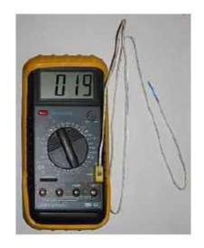
Fig. (4) Thermocouple with display unit.
