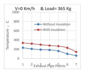
Fig. (9) Temperature distribution at zero car speed and load of 365 Kg.
