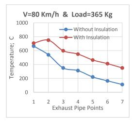
Fig. (15) Temperature distribution at 80 Km/hcar Speed and load of 365 Kg.
