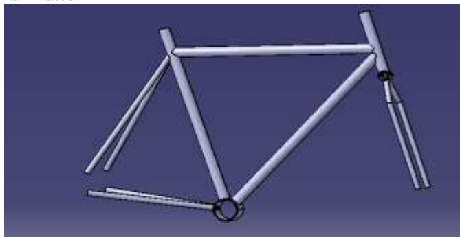
Fig.1: Bicycle model done in Catia software
