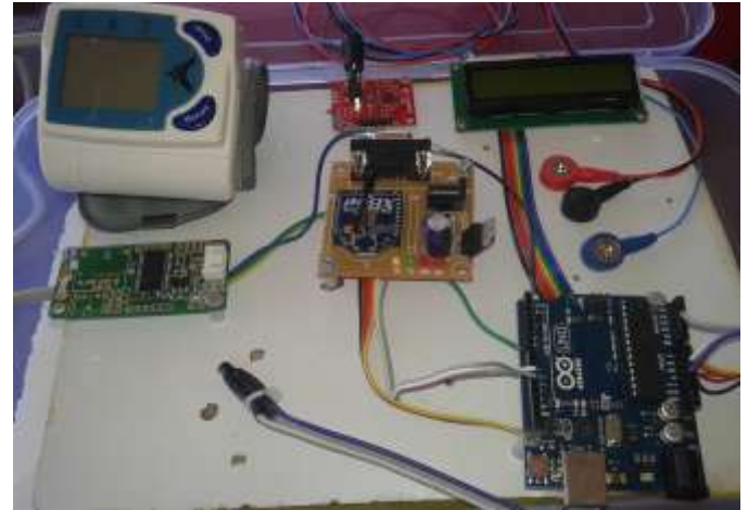
Fig 5. Transmitter hardware with Sensors, MCU, Zigbee.
