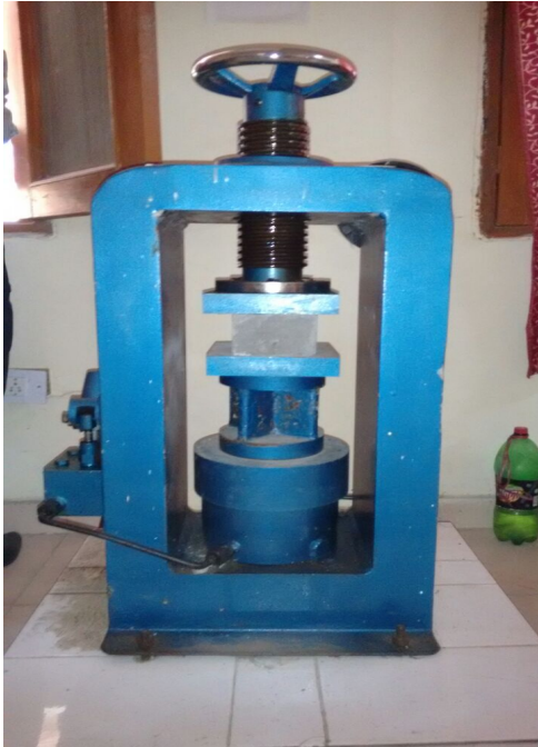
Fig 1: Experimental Setup For Compressive Strength Test
