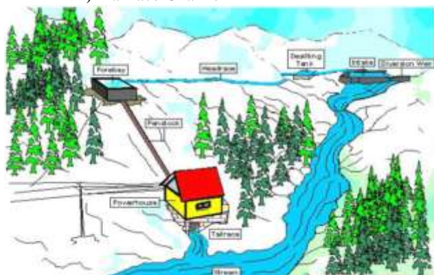
Fig 1. Typical Arrangement of SHP
