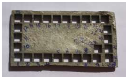
Fig. 3.4 Aluminium metal matrix after machining 10mm slots
