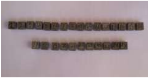
Fig. 3.5 Pieces removed from specimen
