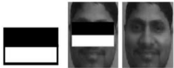
Fig.3.6 Haar Feature that looks similar to the eye region which is darker than the upper cheeks is applied onto a face
