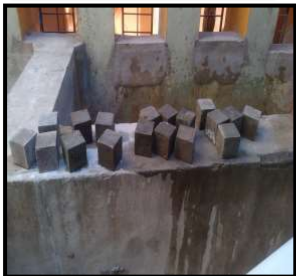
Fig.7 Mortar mixture and Casted Mortar specimen of size 70.6x70.6x70.6 MM 3
