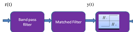
Fig..3.2 Block Diagram Of Matched Filter Detection
