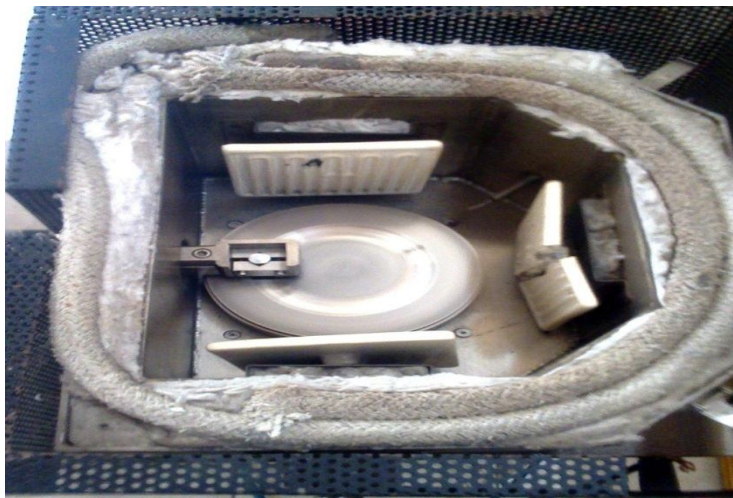
Fig. 2 Close up view of specimen loading in Pin-on-Disc Tribotester
