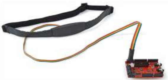
Fig. 7 Position Monitoring sensor to Arduino board
