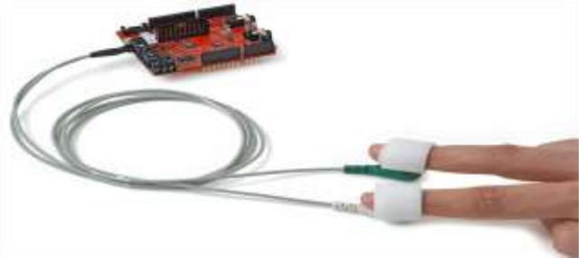
Fig. 8 GSR sensor to Arduino board
