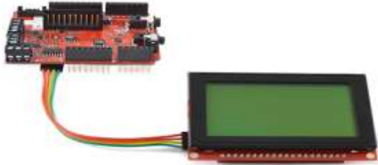
Fig. 11 Graphical LCD attached to Arduino board
