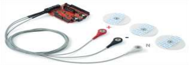
Fig. 3 Electrodes for ECG attached to Arduino board
