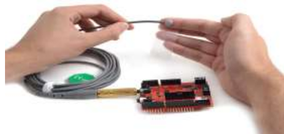
Fig. 5 Body Temperature Mesurer to Arduino board
