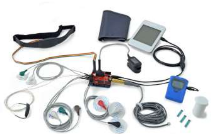
Fig. 1 Modules interfacing with Arduino board
