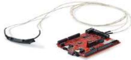
Fig. 4 Airflow mesurement sensor to Arduino board
