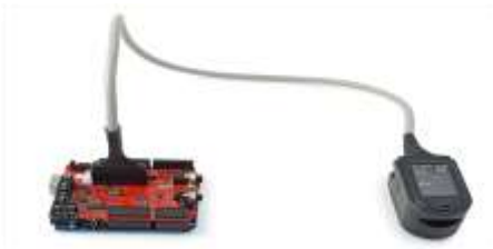
Fig. 2 Pulse and Oxygen Mesurment sensor to to Arduino board
