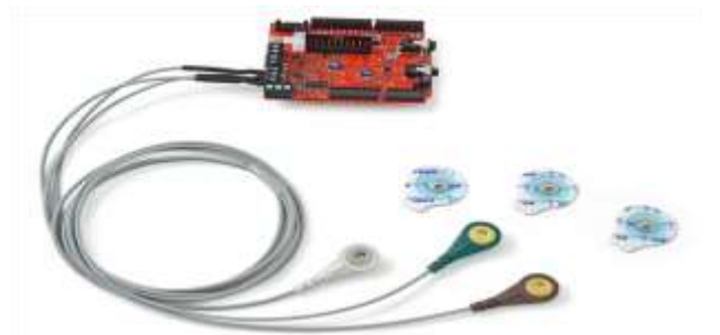
Fig. 10 EMG Sensor attached to Arduino board
