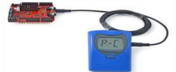
Fig. 9 Glucose mesurer attached to Arduino board
