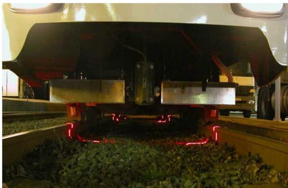
Fig.3: Alignment of Ultra sonic sensors
