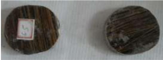
Fig.2. Thermal conductivity testing specimens
