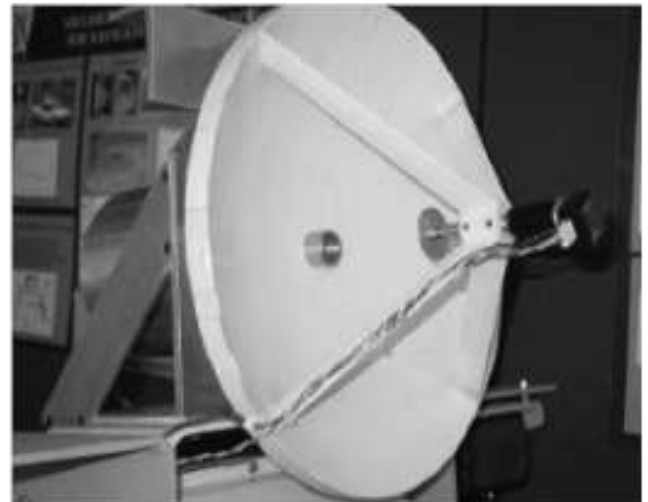
Figure 1 Monopulse feed placed at the focal point of reflector antenna
