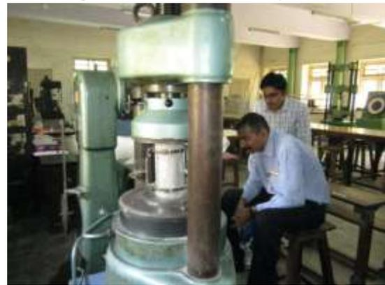
Figure 5: Setup of Modulus of Elasticity Test
