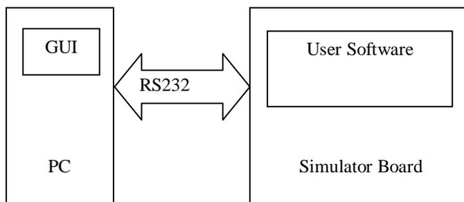
Fig: 1.1 Connection between the GUI and Simulator Board
