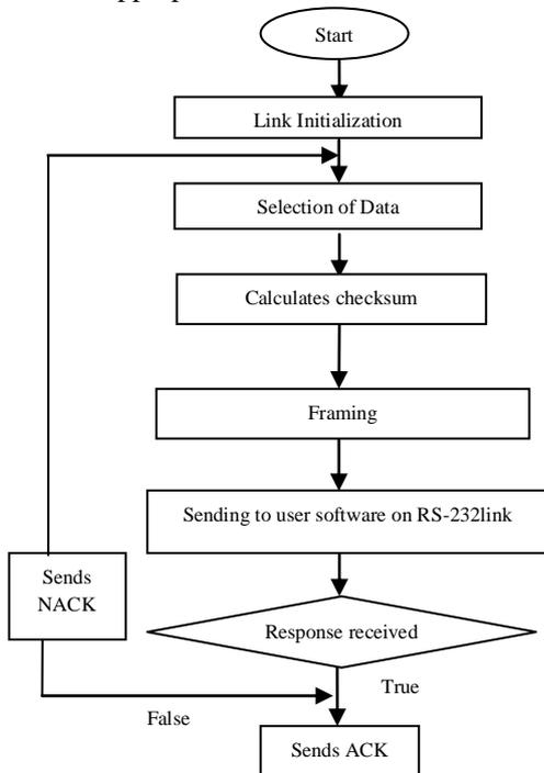
Fig. 2.2 GUI flow diagram
