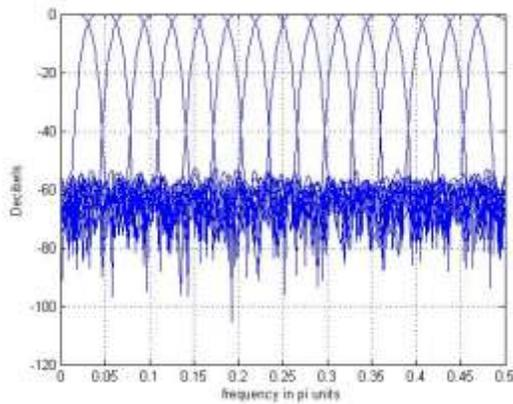
Fig.3 (c) Magnitude response of 16-band analysis filter bank at  $\alpha = 2^{-12}$
