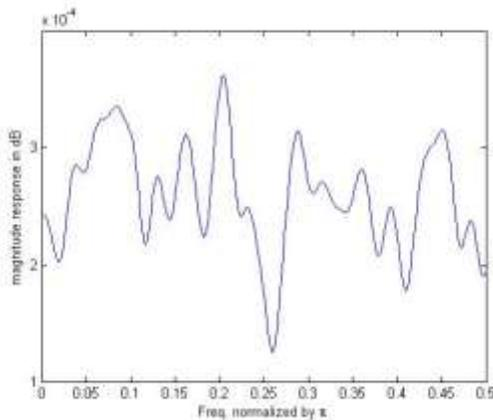
Fig.2 (g) Magnitude response of Aliasing distortion function at  $\alpha = 2^{-12}$
