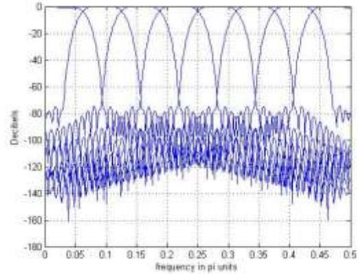
Fig.2(b) Magnitude response of 8-band analysis filter bank
