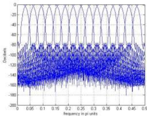
Fig.3 (b) Magnitude response of 16-band analysis filter bank
