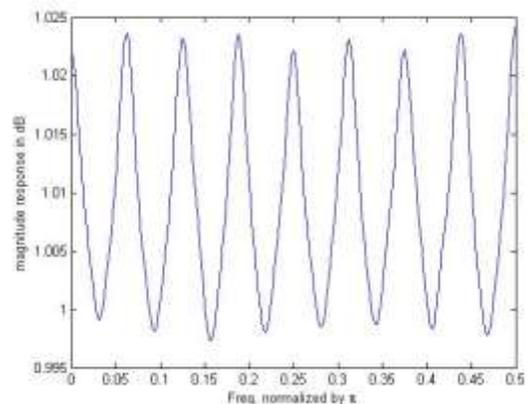
Fig.3 (f) Magnitude response of Amplitude distortion function at  $\alpha = 2^{-12}$
