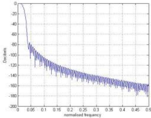
Fig.3 (a) Magnitude responses of optimized prototype filter
