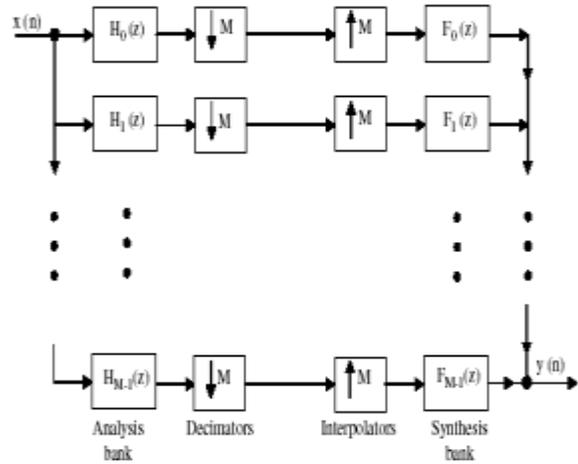
Fig. 1. M-Channel Uniform Filter Bank.
