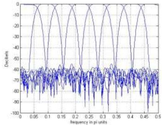
Fig.2 (c) Magnitude response of 8-band analysis filter bank at  $\alpha = 2^{-12}$
