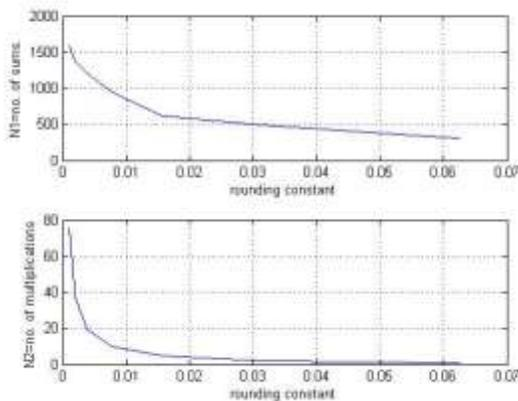
Fig.3 (h) Computational complexity graph for the designed 16 band filter bank according to Table.2
