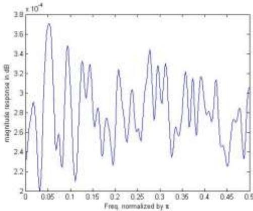
Fig.3 (g) Magnitude response of Aliasing distortion function at  $\alpha = 2^{-12}$
