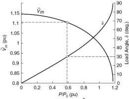
**Figure. 8** The midpoint voltage,  $\tilde{V}$ , and load angle, d, as functions of P / P<sub>0</sub>.
