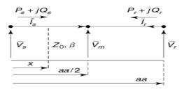
Figure. 4 The power on a lossless distributed line.
