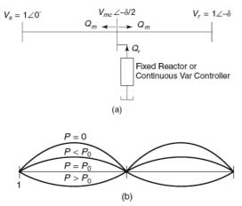
Figure. 9 The midpoint-overvoltage
