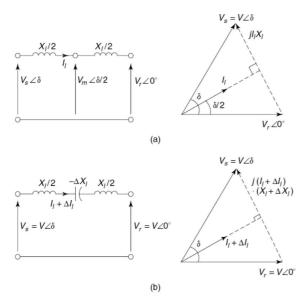
**Figure. 13** The series compensation of a short, symmetrical transmission line.
