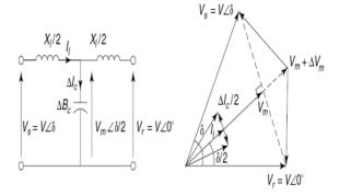
**Figure. 14** The midpoint-capacitor compensation of a short, symmetrical line.
