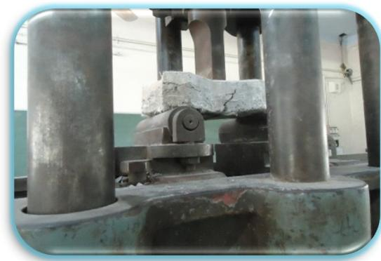
**Figure 5: Setup of Flexural test**
