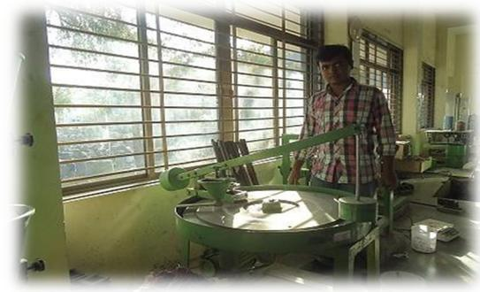
**Figure 4: Setup of Abrasion Resistance test**
