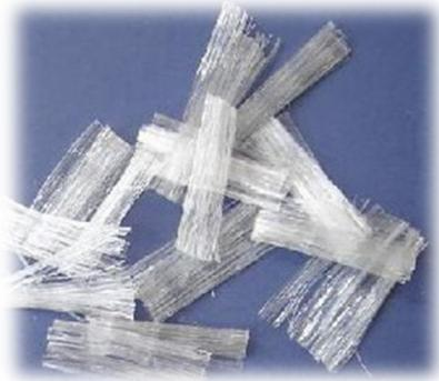
**Figure 2: Polypropylene Fiber**
