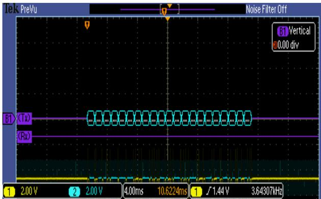
Fig. 10 data from CAN bus to conversion interface
