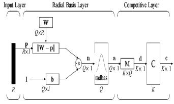
Figure 3. Network Structure, R=5, Q= 1800, K=32
