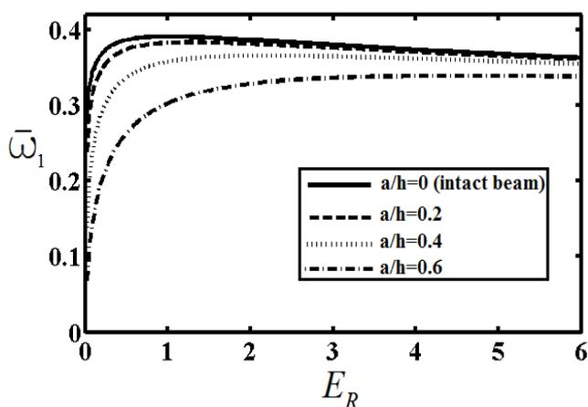
Figure 4 The effect of Young’s modulus ratio  $E_R$  on the dimensionless fundamental frequency  $\bar{\omega}_1$  for different the crack depth ratios  $a/h$ .
