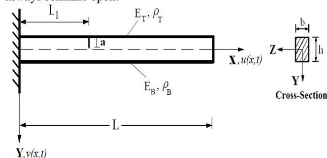
**Figure 1.** A cantilever FGM beam with an open edge crack and cross-section.
