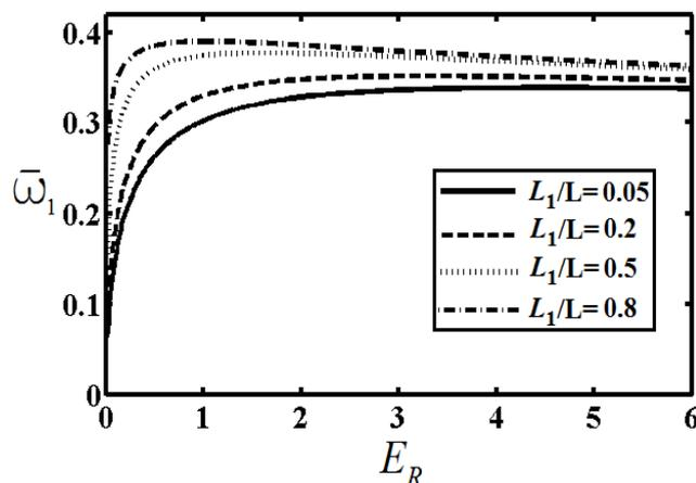
Figure 5 The effect of Young’s modulus ratio  $E_R$  on the dimensionless fundamental frequency  $\bar{\omega}_1$  for various the crack locations ( $L_1/L$ )
