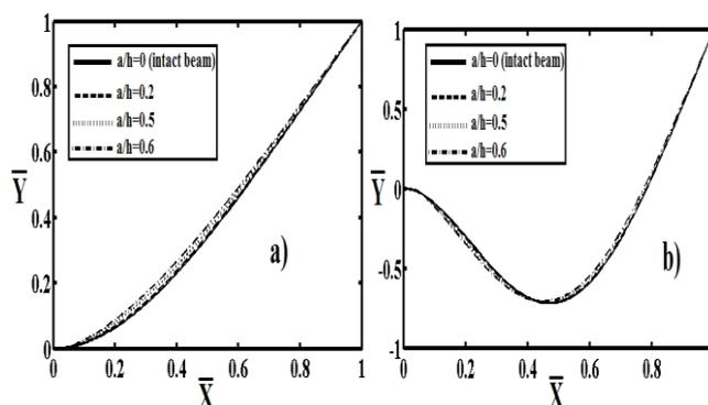
**Figure 8** The effect the crack depth ratio  $a/h$  on the a) first and b) second normalized vibration mode shapes.
