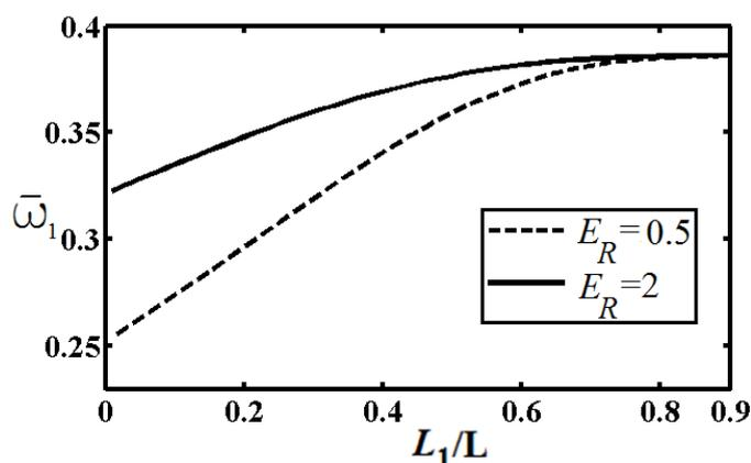
**Figure 6** The effect of crack locations ( $L_1/L$ ) on the dimensionless fundamental frequency  $\bar{\omega}_1$  for  $E_R = 2$  and  $E_R = 0.5$ .
