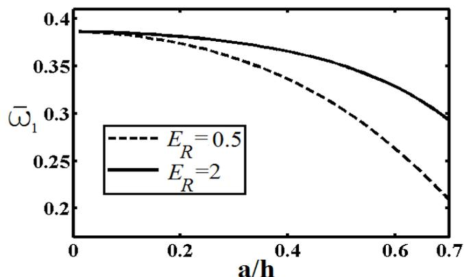
**Figure 7** The effect the crack depth ratio  $a/h$  on the dimensionless fundamental frequency  $\bar{\omega}_1$  for  $E_R = 2$  and  $E_R = 0.5$ .
