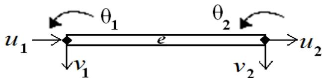
Figure 2. A two-node beam element
