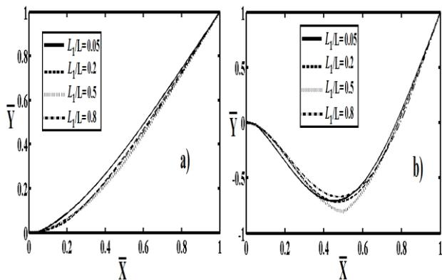
Figure 9 The effect the crack location  $L_1/L$  on the a) first and b) second normalized vibration mode shapes.
