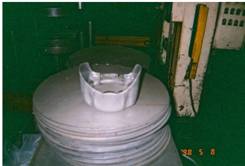
Fig.No.2 (b): Fracture at the side walls
