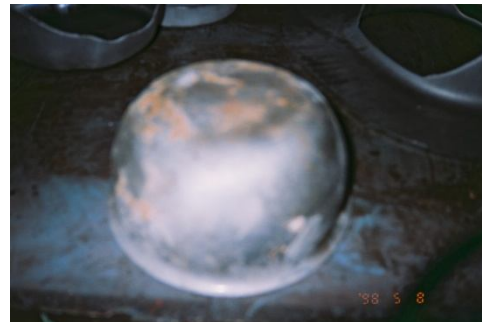
Fig.No.2 (a): Fracture at the bottom of the cup
