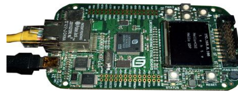
Figure 4: Stellaris TI- EKLM3S6965 Ethernet eval. Board[8]
