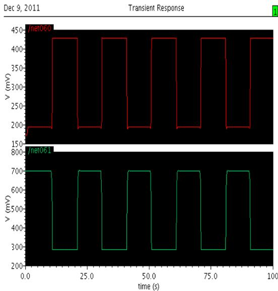
Fig. 8. Output waveform of 8T SRAM cell
