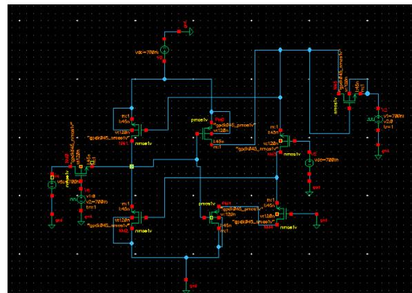
Fig .2. Schematic of 8T SRAM cell
