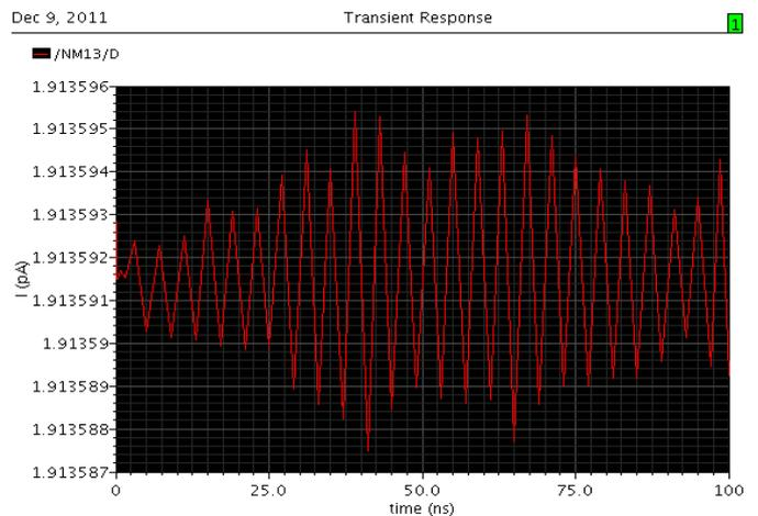
Fig. 11 Leakage current in 7T SRAM cell using AVLS technique.
