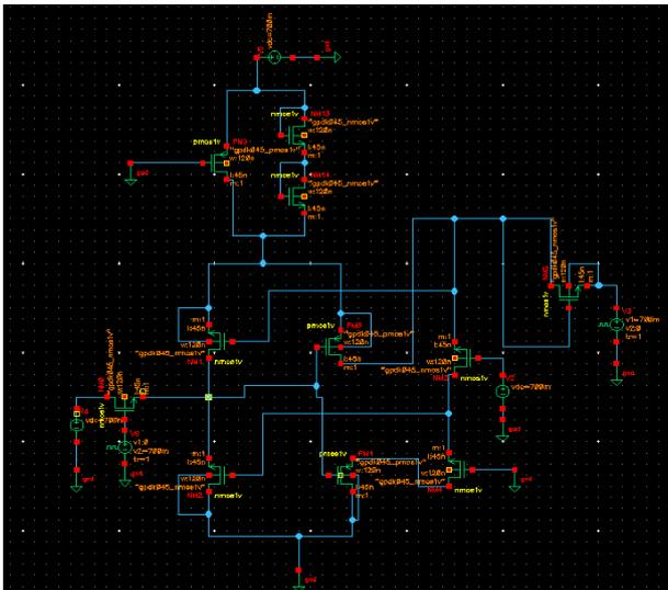
Fig.6. Schematic of 8T SRAM cell using AVLS technique
