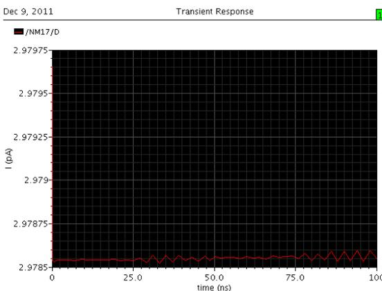
Fig. 10 Leakage current in 8T SRAM cell using AVLG technique.
