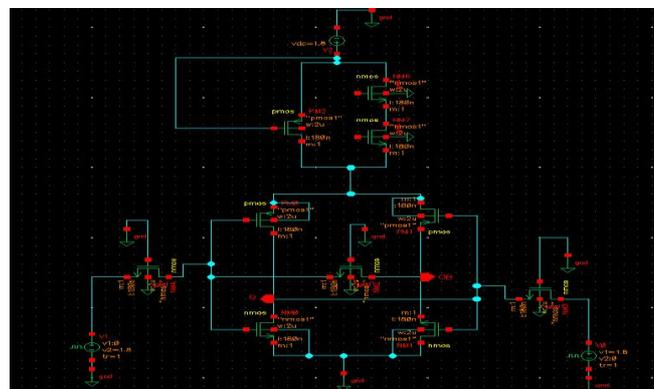
Fig.5. Schematic of 7T SRAM cell using AVLS technique
