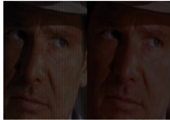
Fig. 2 Difference of quality of display between DK1 and DK2, Left side image is of DK1 and right side image of DK2.
