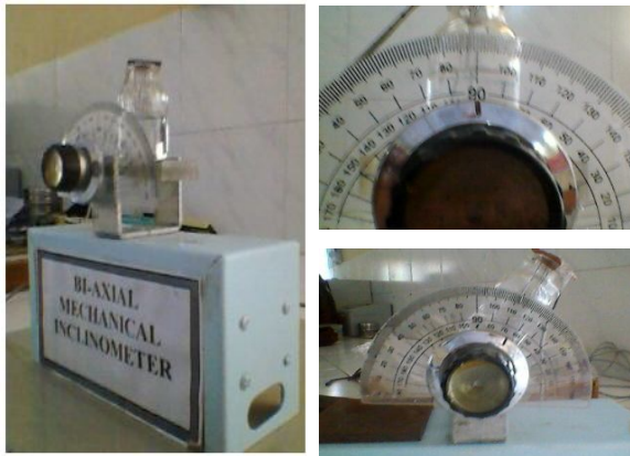
Fig.4. Shows bi-axial mechanical inclinometer for fall angle measurement & right image shows 24 deg fall angle.
