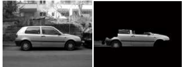
Fig 2. left: Original image, right: segmented image
