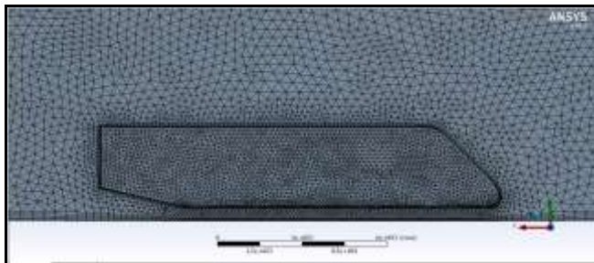
Fig. 2 Meshing of the conceptual bus
