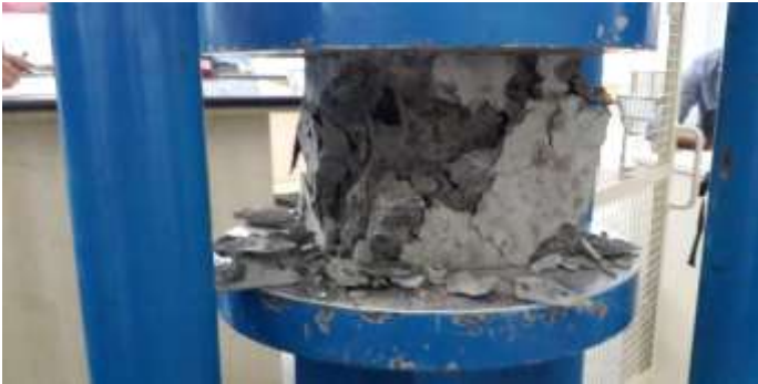
Figure 2: Compression test on Concrete cube
