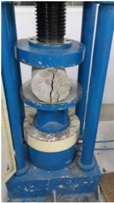
Figure 6: Tensile Strength on Concrete Cylinder
