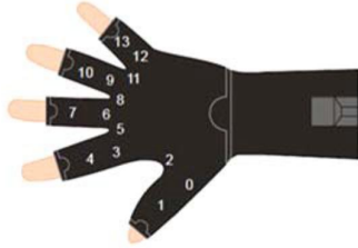
Figure 1. Description of sensors on Data Glove
