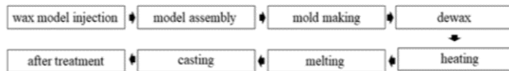
Fig. 1 Steps in the investment casting process for high carbon high chromium white cast iron
