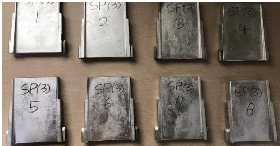
Fig. 8 Research prototype and develop products of high C-high Cr white cast iron blades
