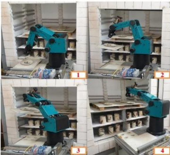
Fig. 6 Articulated Robot Arm Moving of Loading and Unloading a Ceramic
