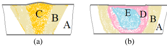
Figure 1. Schemes of the affected zones in the fusion welding processes (a) and in the FSW (b). Source: own.
