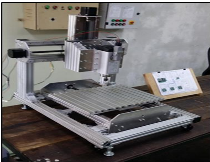
Fig. 6 Machine development and frame structure design
