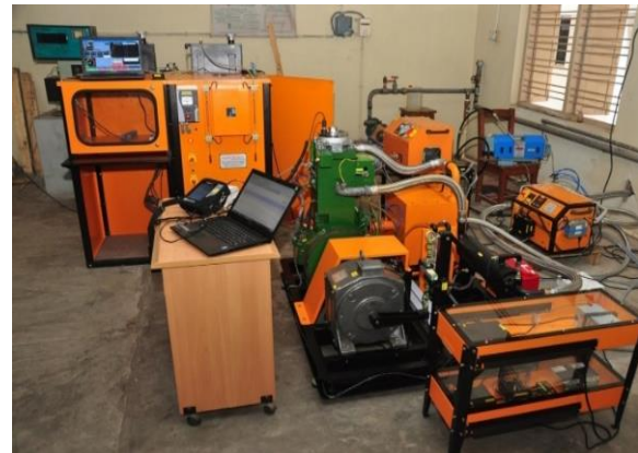
Fig.4. The computerized multifuel high-pressure engine test rig
