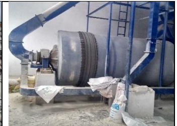
Fig.1b Miller used for crushing of ceramic tiles waste
