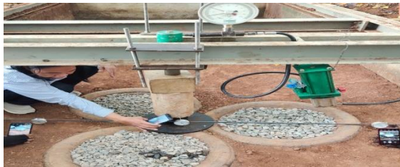
Fig 14 : Horizontally arranged tire foundation model test
