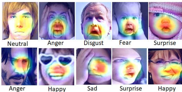
Fig. 6 Activation maps using GRAD-CAM on sample images from RAFDB and AffectNet datasets (predicted expressions are displayed below each image). Red color denotes higher saliency while blue color denotes lower saliency. Yellow color denotes moderate saliency.
