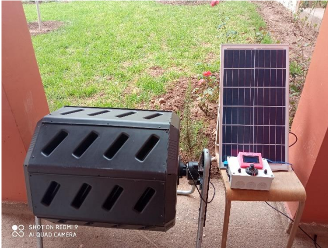
Fig 6: Reel solar composter
