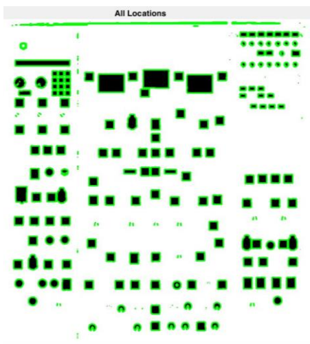
Fig.11. All locations were obtained by conversion of a color image into a Black and White image using the Color Channel-based method.
