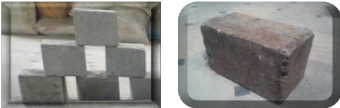
Fig. 6. A Moulded Block of Size 6'' X 8'' X 12'' and With LWC Cubes.
