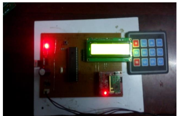
Figure 14. Hardware implementation of Base Station in WSN.
