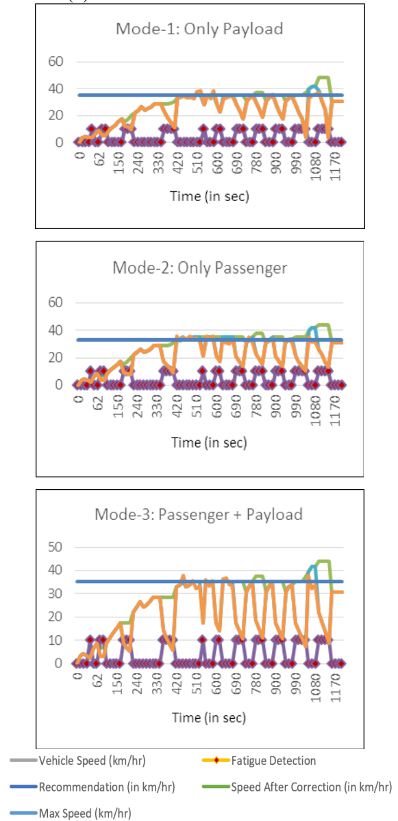
Fig.10 Speed Control due to Fatigue Detection
