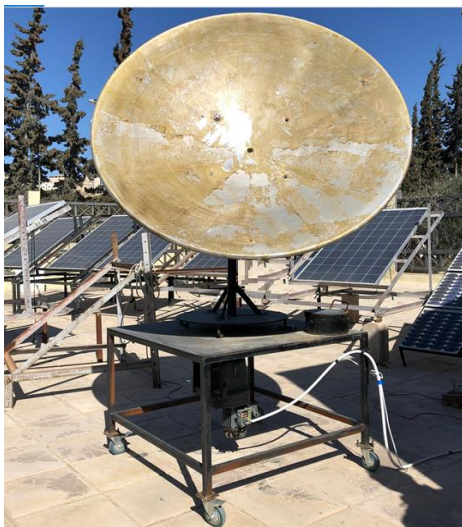
Fig (2). Front view of SSC after manufacturing and without reflecting mirrors
