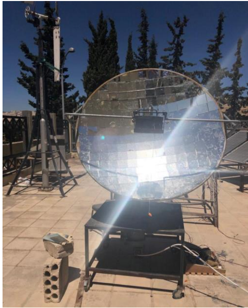
Fig (6). Semi-Spherical solar oven with auto single-axis sun following system
