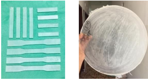
Fig.3.1 Casting Slabs and Mechanical Test Objects
