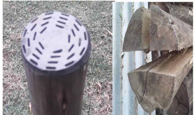
Figure 3- End plate used to prevent the splitting end
