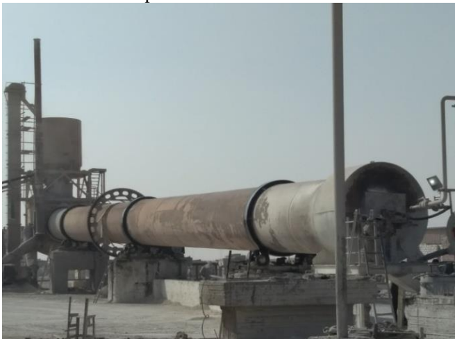
Fig. 4: Horizontal Rotary Calcination Kiln
